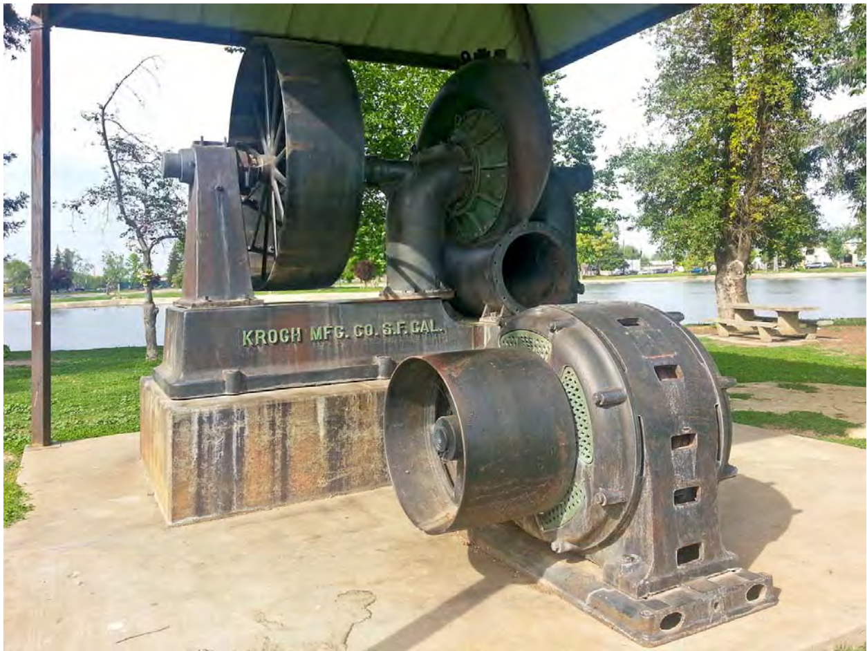
Figure 4. In 1895 Pumps were installed at the confluence of the Yuba, and Feather Rivers, to protect the city of Marysville from the danger of flooding and were powered by high capacity electric motors.
