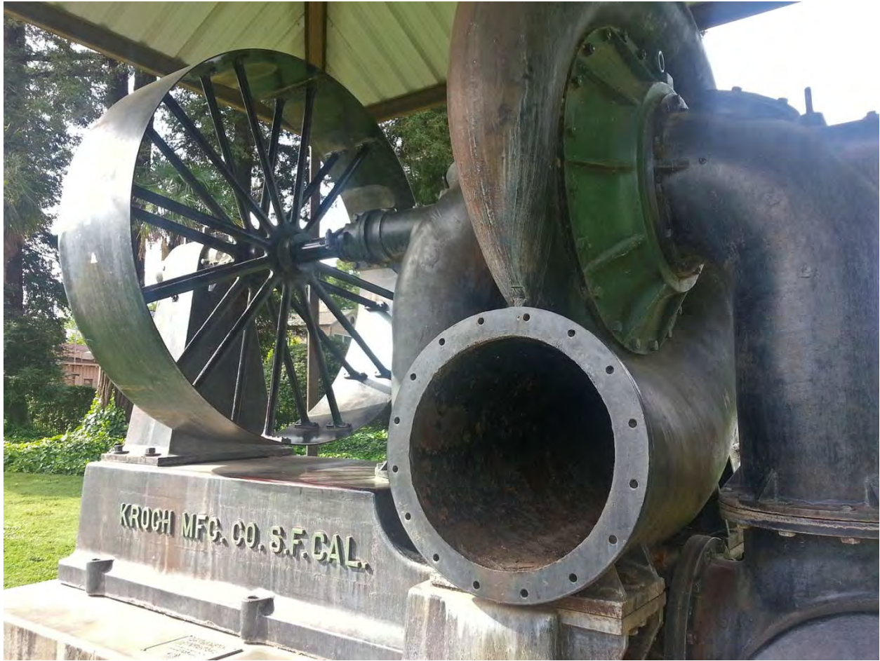
Figure 5. These pumps have a capacity to pump 18,265 gallons per minute. That's approximately equal to the capacity of the average back yard swimming pool, each minute.
