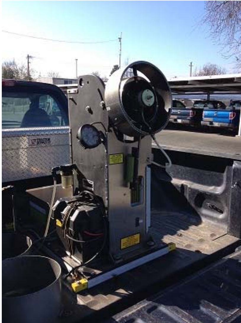
Figure 1. An example of a SYMVCD fogger unit. (January 2015)
